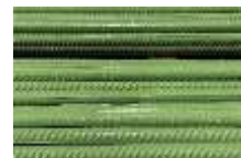
Epoxy coated TMT bars
